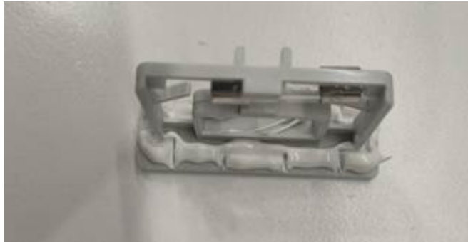
Figure 7-49 Taking out the fuse box
