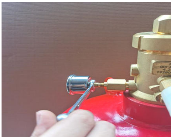
Figure 2-6 Tightening the pressure gauge
