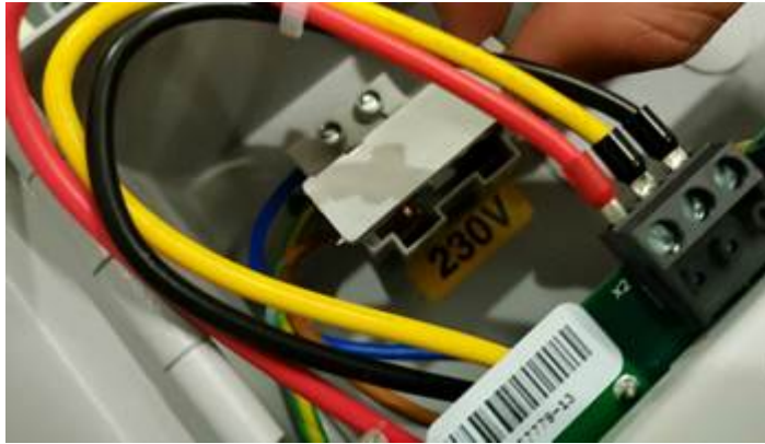
Figure 7-51 Installing the fuse box
